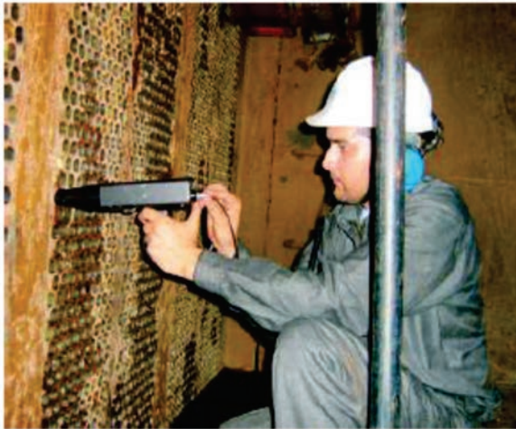
Fully covering the tube opening to block any external noise picked up by equipment
