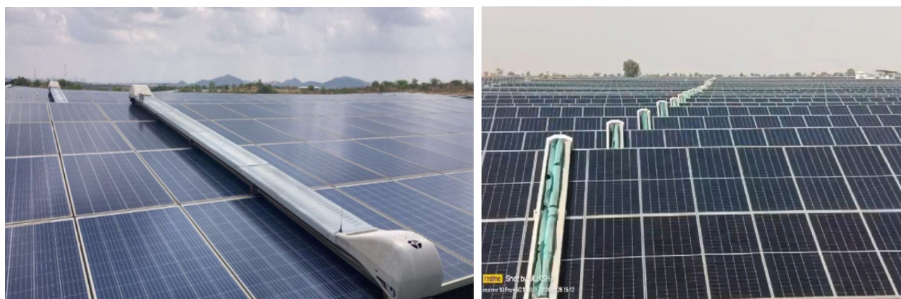
Figure 1: Robotic dry cleaning of solar modules in Ground Mounted Solar project
