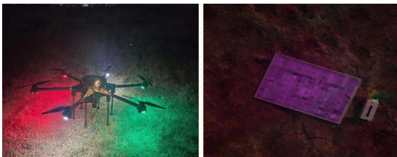
Figure 7: EL Testing of Solar plant
