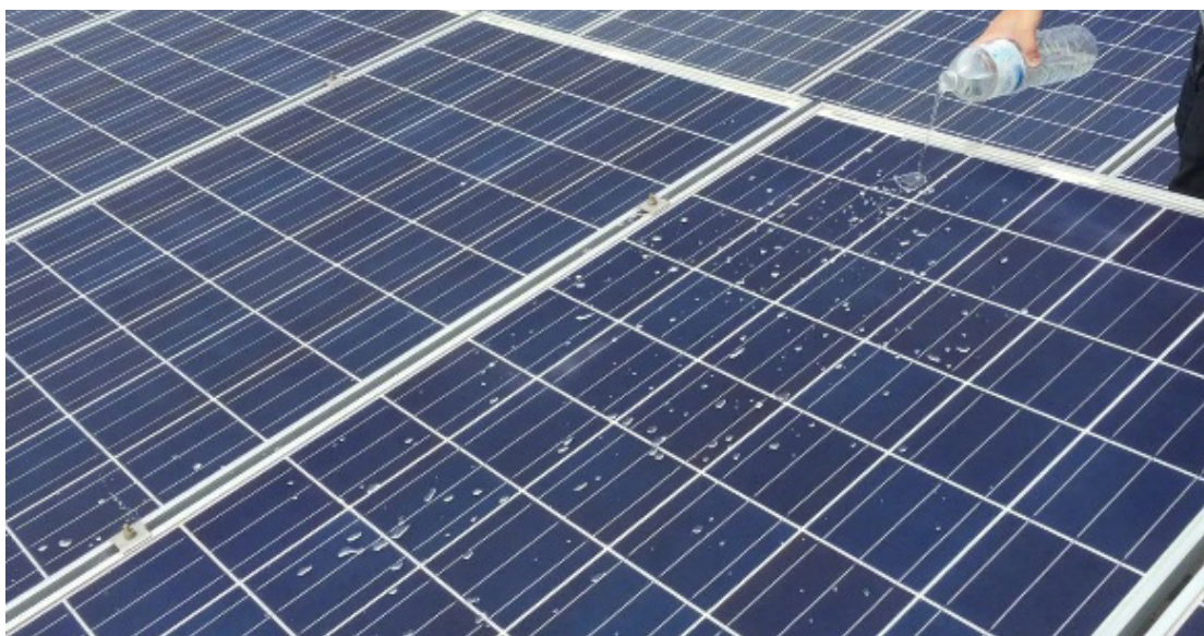
Figure 6: Solar module with nano coating
